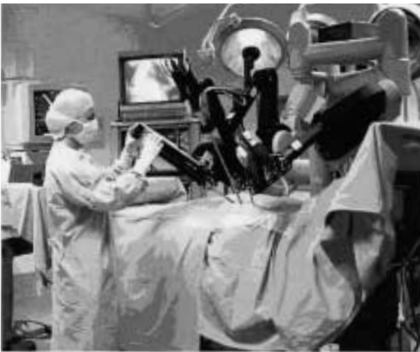
Figure 2. The robotic unit with the endoscope and the surgical instruments.
