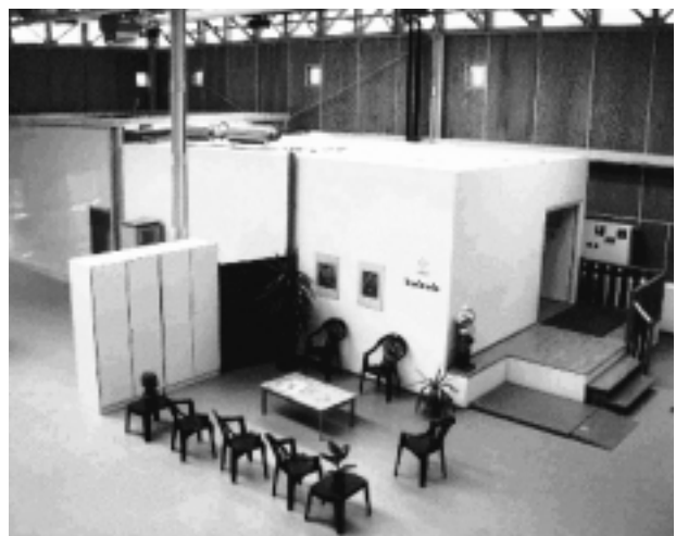
Figure 1. Magnetically shielded room installed at the University of Ulm (Germany).
